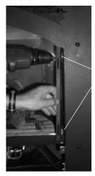
Door Bracket attaches with 2 screws.
